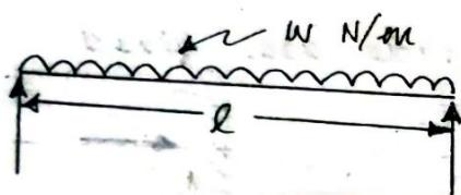
$l \rightarrow$  span of the beam or distance b/w supports
